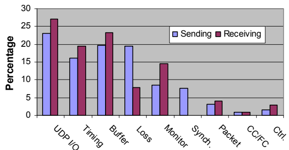
Figure 4. UDT CPU utilization by functionalities. The functionalities listed above include UDP IO, Timing, buffer and memory operation, loss list access, performance and statistics monitoring, synchronization between threads, data packing/unpacking, congestion/flow control, and control message processing.
